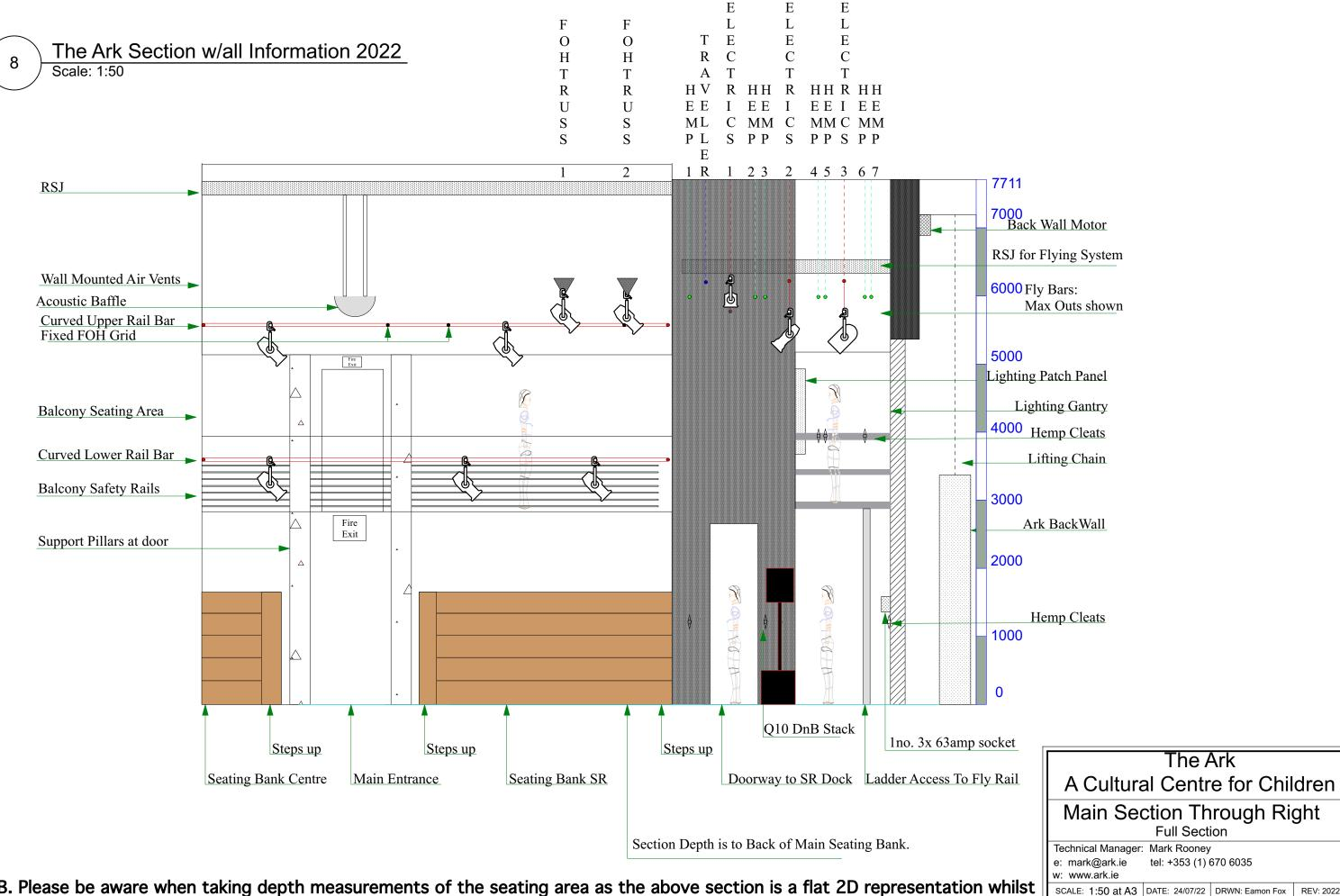
N.B. Please be aware when taking depth measurements of the seating area as the above section is a flat 2D representation whilst the seating bank is in reality an arc. Dimensions will not match to the reality.
